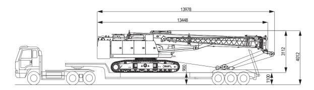
■ Transportation mode II: dismantle the counterweight,transport through two vehicles with maximum weight of single piece transportation 31t, 13.40m×2.99×3.11m (L x W x H)
